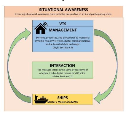
These considerations are interrelated and are critical to monitor and manage ship traffic comprising a mix of conventional, automated and autonomous ships to ensure the safety and efficiency of ship movements through the provision of information or issue advice, warnings, and instructions.
